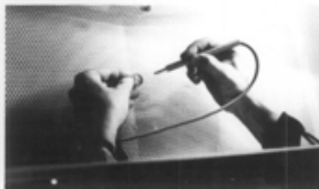
Micro-Abrasive Cleaning. This small, pencil-sized micro-abrasive unit is used by some museum conservators to clean small objects. This particular micro-abrasive unit is operated within the confines of a box (approximately 2 cubic feet of space), but a similar and slightly larger unit may be used for cleaning larger pieces of sculpture, or areas of architectural detailing on a building. Even a pressure cleaning unit this small is capable of eroding a surface, and must be carefully controlled.
