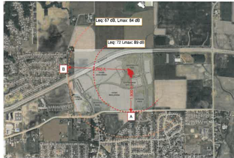
Figure 4: Sound Level Contour Map of Projected Sound Levels from Amphitheater to Neighboring properties
