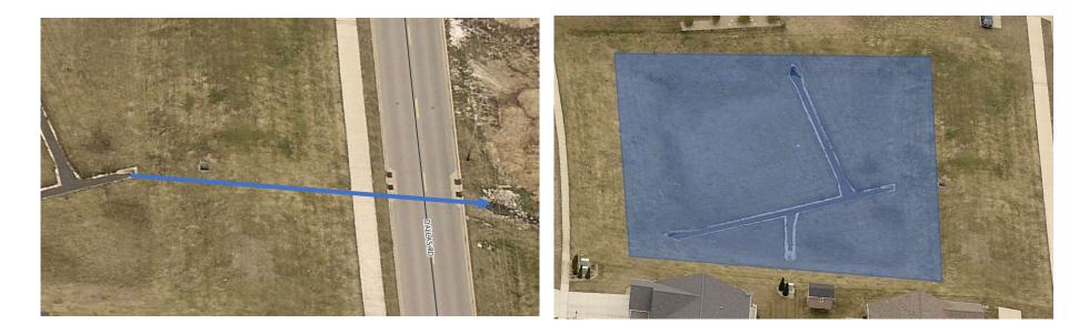
Storm is controlled and reduced to pre-development low flows. Increase in channel flows from surrounding properties is just as impactful as that from basins. Basins will continue low flow after the storm has expired.
