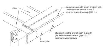
5 RIM JOIST CONNECTION DETAIL NTS
